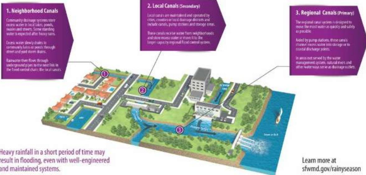
Heavy rainfall in a short period of time may result in flooding, even with well-engineered and maintained systems.
